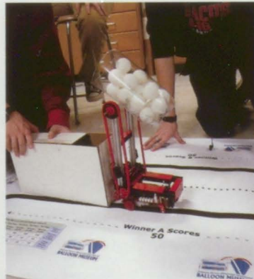
This robot has been programmed to follow the line on the paper that has been placed on the floor and dump the ping pong balls into the box at the end.
